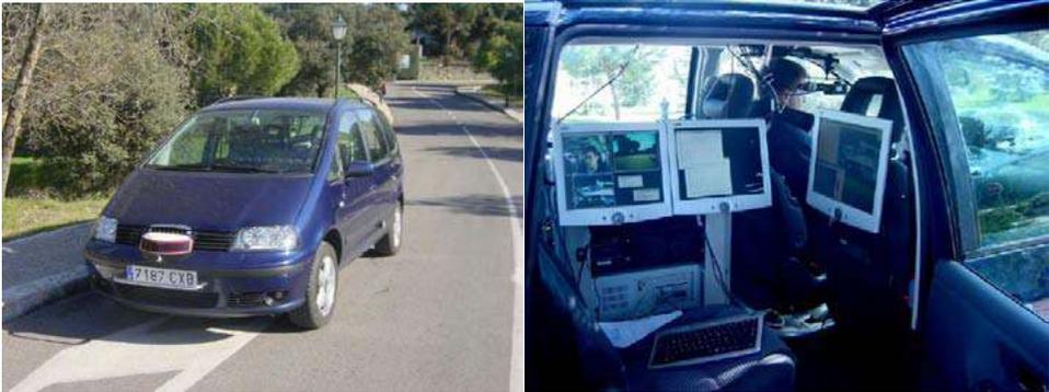
Figure 1. The ARGOS car; left the outside view and right the insight view of the equipment in the back
